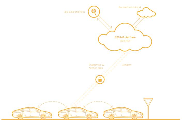
Not only does the CES IoT platform help to control and optimize the complex information flow, it also acts as the interface between human, machine and the Internet of Things.
